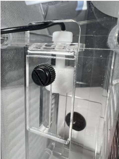
Fig. 2: Mounting the float switch (height adjustable using a screw)
