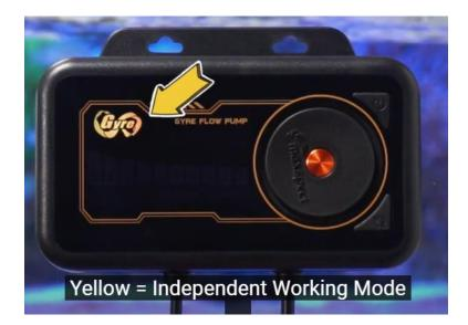
1-1) If the logo is with the yellow color, it means the controller is on the Independent Working Mode, then we can go to Step 2);
