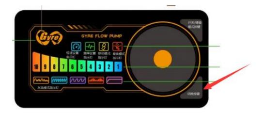
Press the switch button for 3 seconds, it goes into working mode status; Press again the switch button, it changes the working mode, when the logo color turns yellow, meaning it is on the Independent Working Mode, then press the switch button for 3 seconds to save the mode setting.
